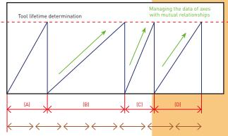
A graph created showing the dispersion of lifetime due to a wide range of reasons in machining. Management based on the short tool lifetime data makes it possible to achieve more stable production.
