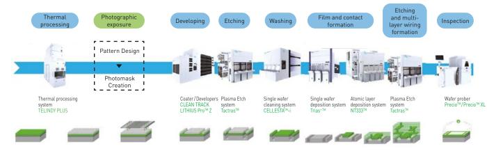
[Fig. 3 Semiconductor manufacturing (Front-end Process) and equipment]
