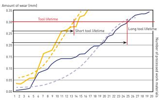
A graph created of tool life based on the acquired data and analysis results. Contributed to the reduction of tool replacement.
